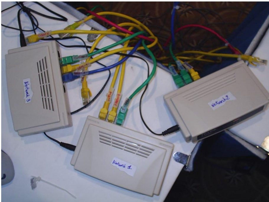
Figure 3.5: IPv6 Core Protocols, Interoperability suite Phase II, test 1.6.D network layout, GNU/Linux router
