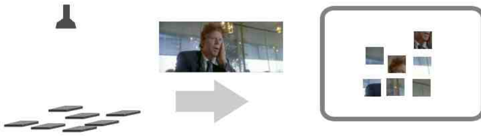
Figure 20 - The camera acquires the pieces' positions and the system then renders the augmented image with the decomposed frame.
