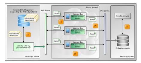
Fig. 1: OVAL-based vulnerability assessment framework for the Android platform
