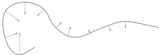
Figure 2.5: Curve with vectors indicating the term \kappa \vec{\mathcal{N}} .
