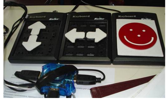
Figure 2. Accessibility switch that allows the user to move the mouse pointer.
