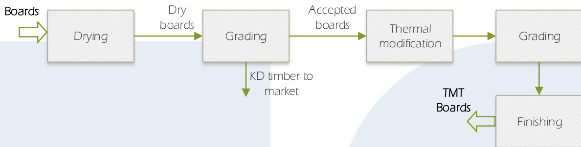
Figure 11. Schematic flow chart of TMT production
