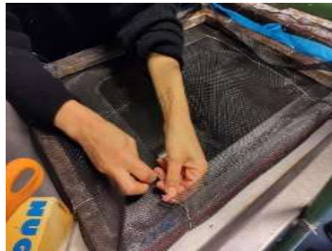
Figure 5. Rack preparation with a metal frame
