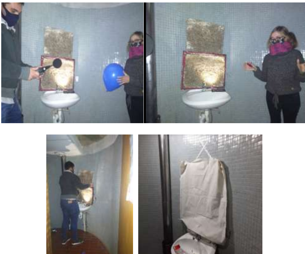
Figure 8. Measuring T_R in a bathroom for testing panels absorption (without and with covering by a piece of canvas)
