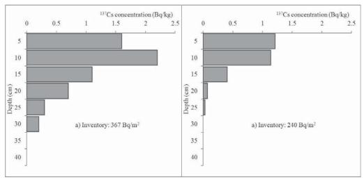
Image 4 – Comparison of <sup>137</sup>Cs profiles associated with soil samples collected from a) reference site, and b) middle slope site in Santo Tomás 1.
