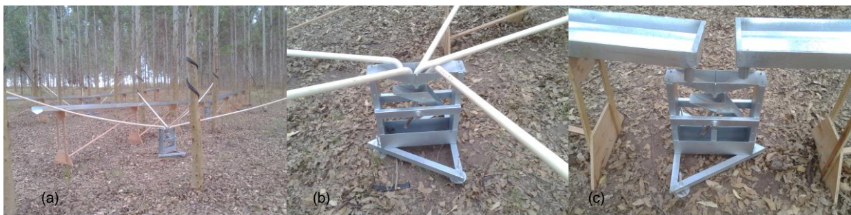
Figure1. (a) The equipment comprised four stationary collectors with gauge system, four collectors troughs and ten collectors for the rubber collar of the threes. (b) stemflow gauge system and (c) throughfall gauge system both of them comprised with a tipping bucket mechanism equipped with actuator, switch output.
