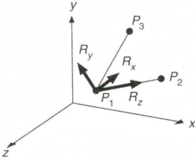
$$R_z = \frac{P_1P_2}{\|P_1P_2\|} = \begin{pmatrix} r_{1_z} \\ r_{2_z} \\ r_{3_z} \end{pmatrix}$$
