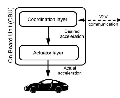
The coordination layer computes the platoon control law using data read from on-board sensors and received from other vehicles through V2V communication
