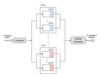
Fig. 2. ATERR Queuing Structure with the Classifier and the Scheduler.
