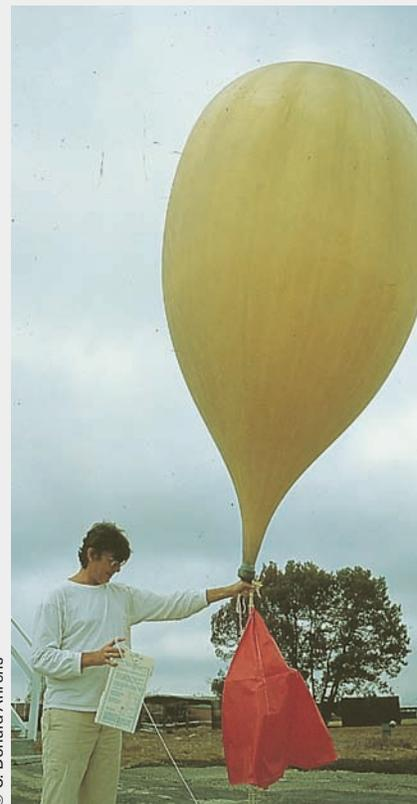
**FIGURE 1** The radiosonde with parachute and balloon.
