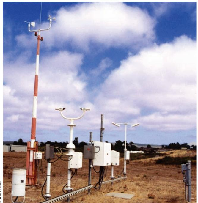
FIGURE 3.18 The instruments that comprise the ASOS system. The max-min temperature shelter is the middle box.
