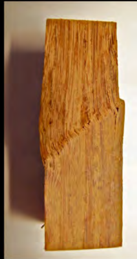
Compression parallel to grain
