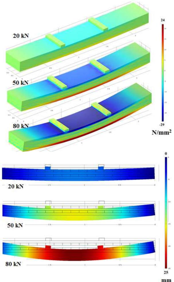
Figure 7. Longitudinal stresses (upper side) and deflections (down side) in the FE model
