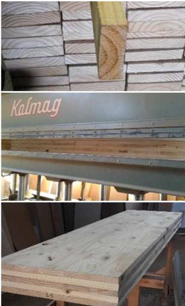
Figure 1. Manufacturing process of a 5-layers prototype of CLT panel
