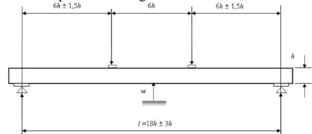
Figure 3. Bending test configuration for sawn timber
