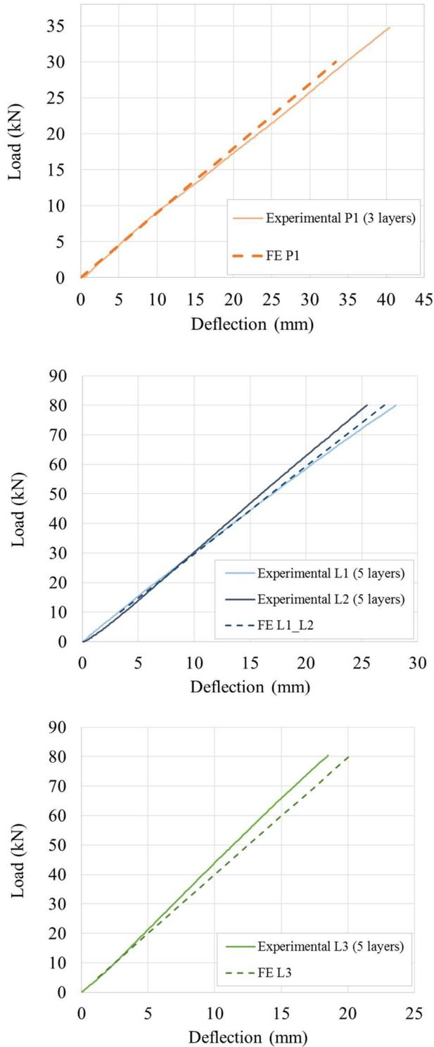
**Figure 8.** Load-deflection curves for experimental and numerical results
