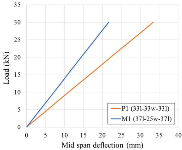
**Figure 10.** Load-deflection diagram for numerical results of different 3-layer panel configurations (M1 and P1).
