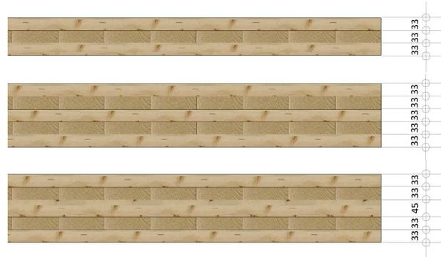
Figure 2. Layer thickness of CLT panels
