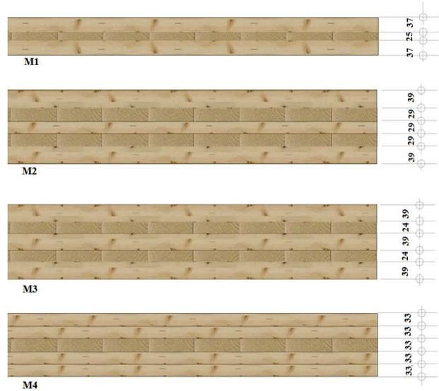
**Figure 9.** Alternative layer configuration evaluated through FE numerical modelling
