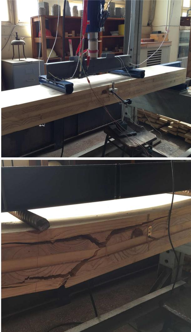
Figure 5. Bending test of CLT panels
