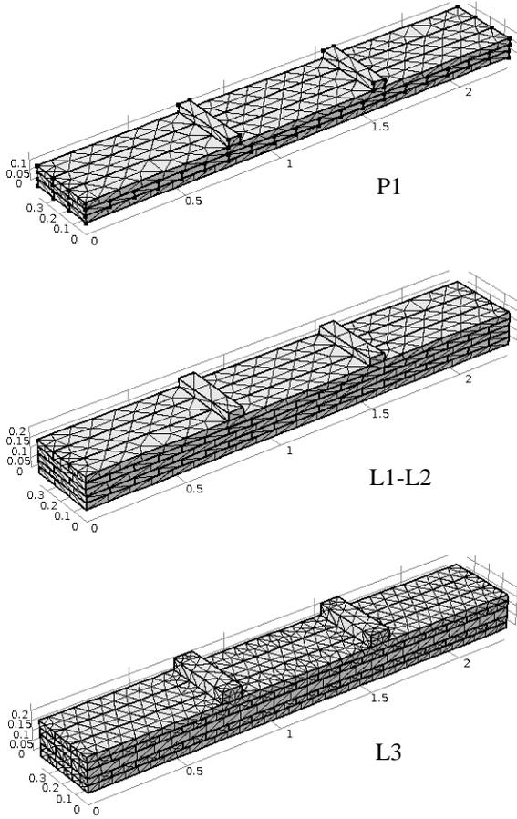
Figure 6. FE model of CLT prototypes
