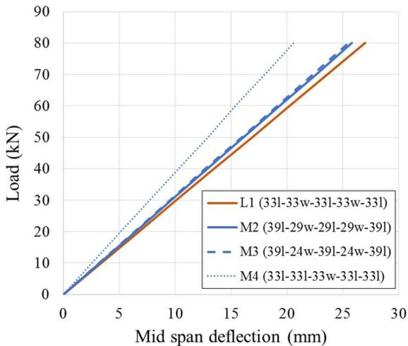
**Figure 11.** Load-deflection diagram for numerical results of different 5-layer panel configurations (M2, M3, M4 and L1).
