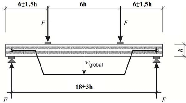
Figure 4. Bending test configuration for CLT prototypes panels
