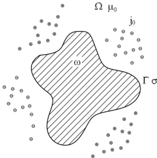
We assume that the electric current frequency is so high that the magnetic field penetrates a negligible distance into the liquid metal (skin effect).
