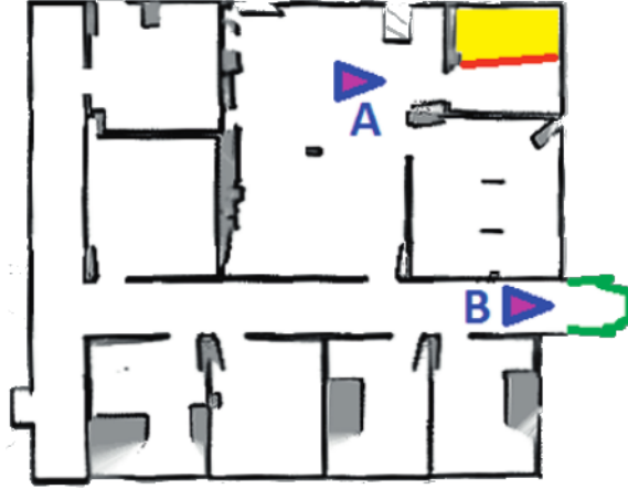
Figure 1.4: Re-exploration caused by restricted communication. (Amigoni, Banfi, and Basilico 2017). The yellow portion of the map is only known by robot B. Thus, robot A goes to re-explore the region beyond the red frontier.
